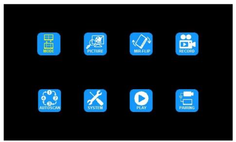
(1) Press  $\triangleleft$  or  $\triangleright$  to select MODE. Press OK to enter. Press  $\triangleleft$  or  $\triangleright$  to select SPLIT/QUAD mode. Select OFF to exit SPLIT/QUAD mode. Press MENU to return to main menu.
